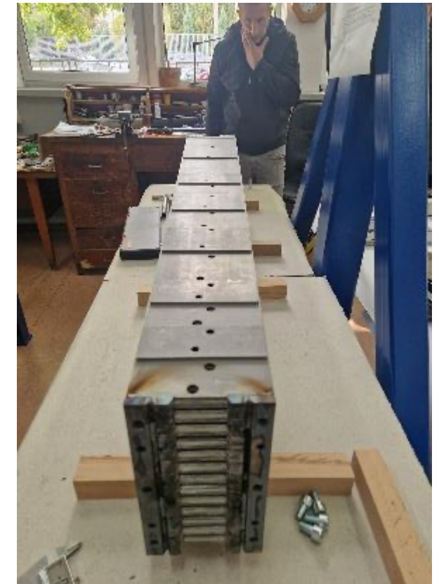
Submodule – 13 periods glued and welded
