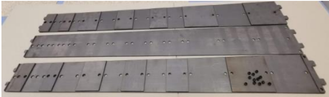
Master and spacers plates for a module period (4 layers)
