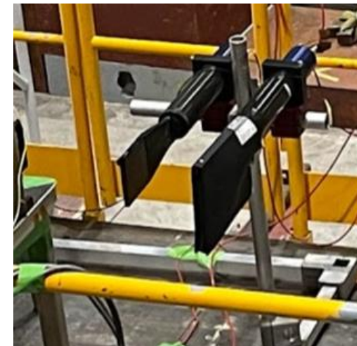
Scintillation counters: Measure the beam intensity
